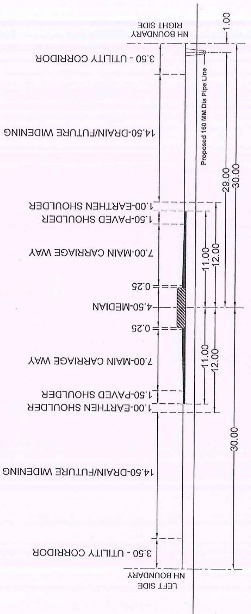
**CH:97/000 TO 97/435 (RHS - WATER PIPE LINE) ROAD CROSS SECTION**
